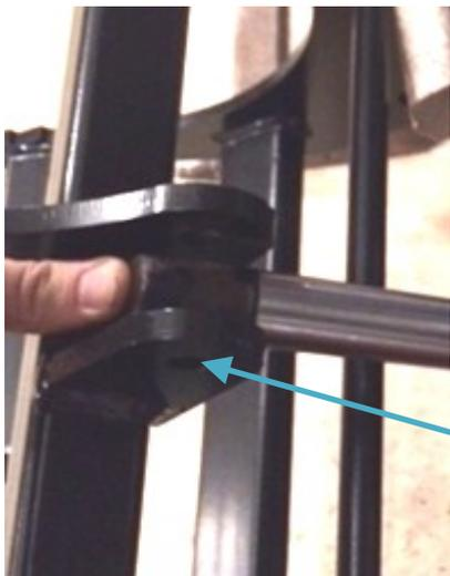
Use the supplied cotter pins to secure these pins to the grapple.
